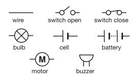
When getting the children to draw circuits, these should be completed with a ruler to make square circuits, rather than free-flowing wires. The positive end of the cell (single battery) is the longer line. A series of single batteries (cells) makes a 'battery'.
